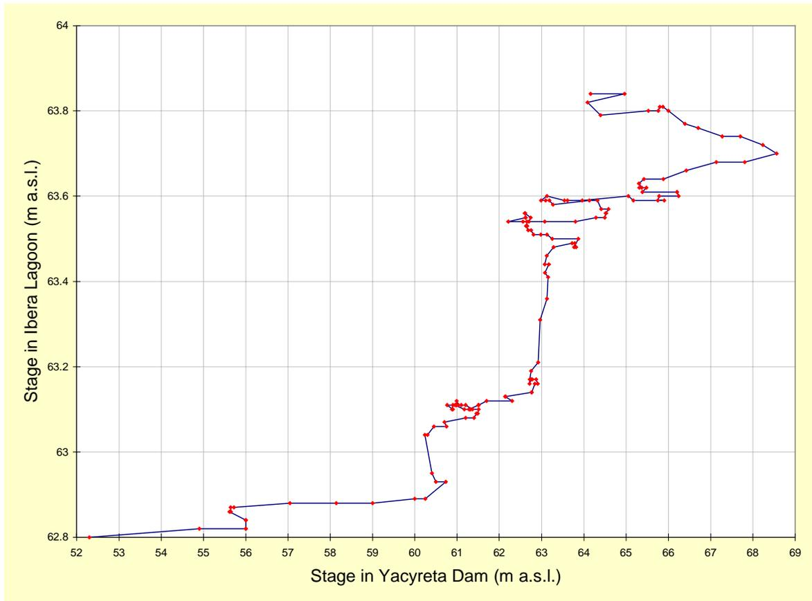
Figure 54. Water level at Ibera Lagoon relative to water level of the Paraná River at Yacyreta Dam.
