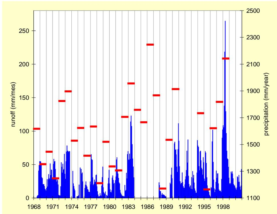
Figure 49. Annual precipitation depth (regional scale) in red and monthly mean runoff across Paso Lucero stream gauge station in blue.
