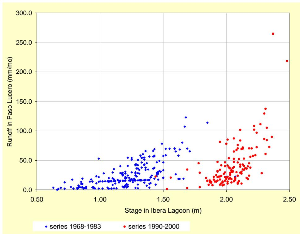
Figure 51. Discharge at Paso Lucero relative to water levels at Ibera Lagoon
