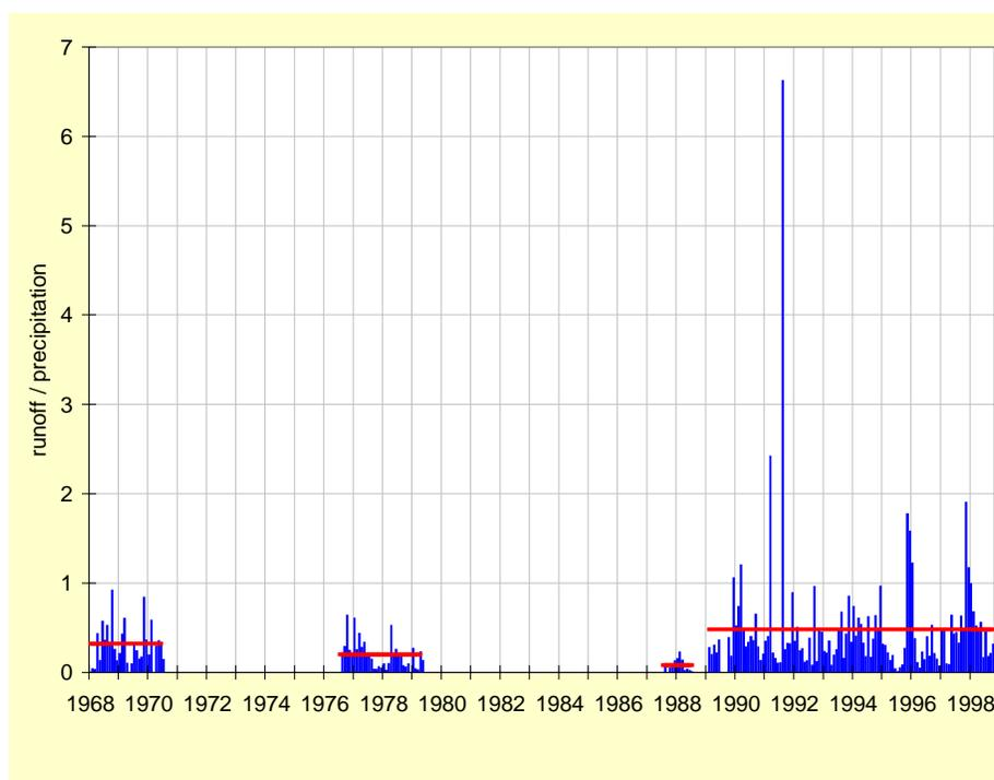
Figure 50. Runoff at Paso Lucero relative to antecedent precipitation.
