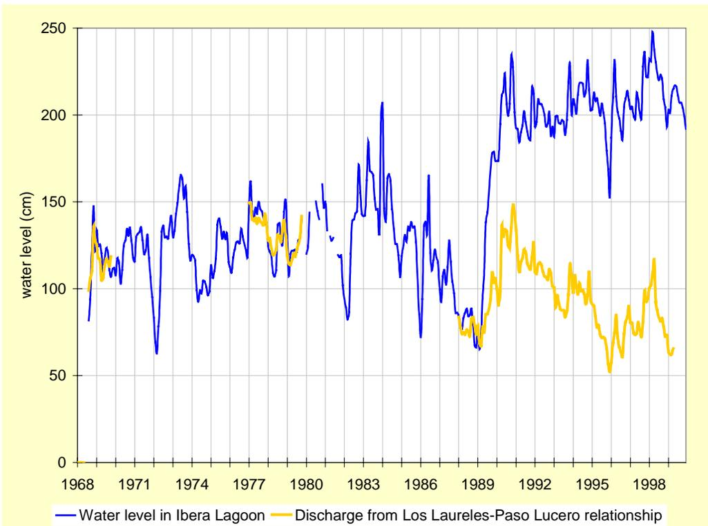
Figure 46: Water level variation in Ibera Lagoon and calculated values considering discharge interpolated from Los Laureles-Paso Lucero relationship in missing data
